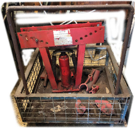
Pipe Bender, Trolley and Metal-craft Master Rolling - Bending - Riveting Tool
